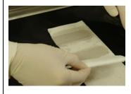
4) Place moist cleaning cassette in drawer. While holding down the **Eject** button, slowly move the drawer in and out 10 times.
