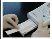
Use the "tape tail" attached to the cleaning cassette to pull the drawer out while holding down the Eject button.
