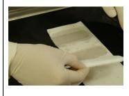
4) Place moist cleaning cassette in drawer. While holding down the **Eject** button, slowly move the drawer in and out 10 times.
