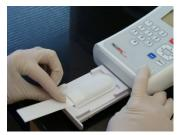
Use the "tape tail" attached to the cleaning cassette to pull the drawer out while holding down the Eject button.
