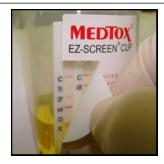
9. Remove the privacy tab and read the results. Control line (C) must be present to read results.
